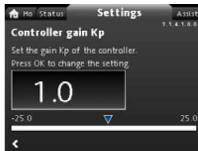
Fig. 59 "Controller gain Kp"
